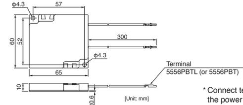
\* Connect terminals to pins No. 3 and No. 5 of the power supply connector, respectively.
