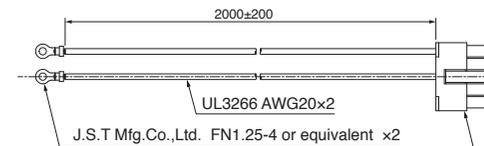
Connector for power supply connection (Molex.)
