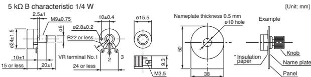
\* Insert the insulation paper to positively isolate the terminals and chassis.
