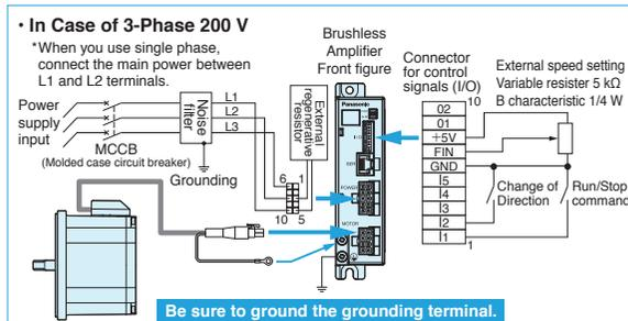
In wiring to power supply (outside of equipment) from MCCB, use an electric wire of 1.6 mm diameter (2.0 mm<sup>2</sup>) or more both for main circuit and grounding. Apply grounding class D (100 Ω or below) for grounding. Do not tighten the ground wires together, but connect them individually.
