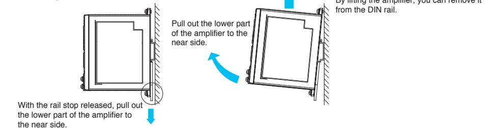
With the rail stop released, pull out the lower part of the amplifier to the near side.
