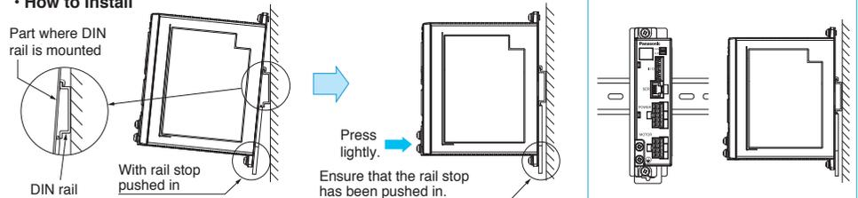
Hook the upper side of DIN rail mounting part on the DIN rail.
